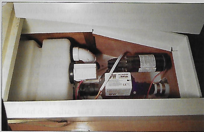
The freshwater plumbing for the sink and toilet is hidden in the bow and beneath the hinged lids of the V-berth.
